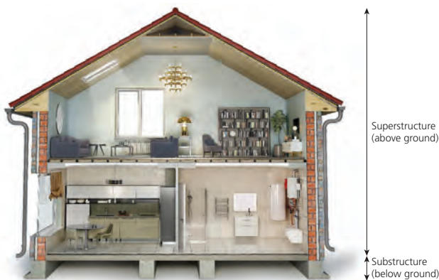
▲ Figure 3.1 Superstructure and substructure of a building
