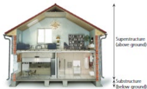
▲ Figure 3.1 Superstructure and substructure of a building
